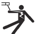
The machine must be connected to an earthed electrical supply. Use the recommended fuse size. An electrical discharge can directly or indirectly cause serious accidents, or death .
