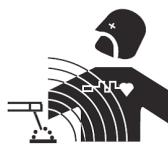
The electric currents flowing through a conductor cause electrical and magnetic fields (EMF). All welders should use the following guidelines to minimize exposure to the welding circuit's electromagnetic fields:
